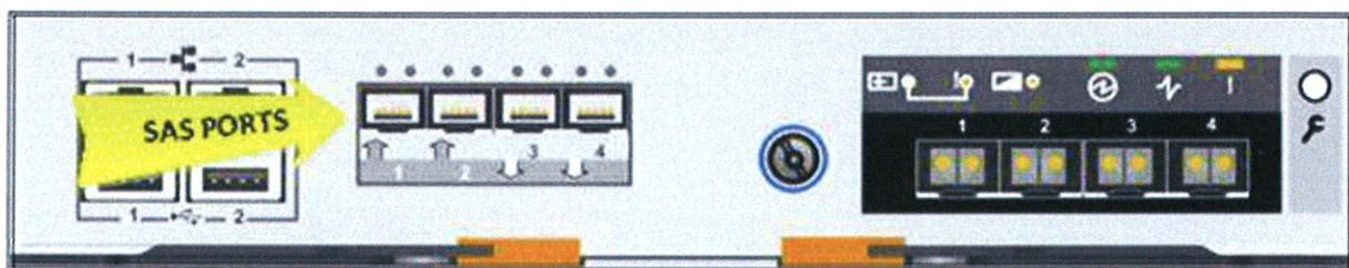
Figure 12-5 Node canister SAS ports
